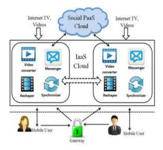
Figure 1: Architecture of Cloud MOV
